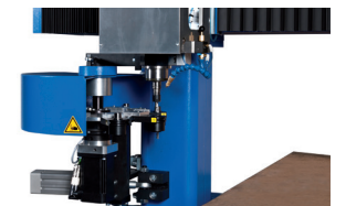
Tellerwechsler 8-fach, optional 8-time Disk type tool changer, optionally
