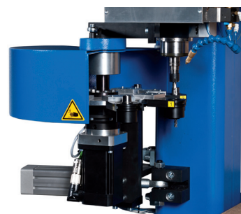
Tellerwechsler 8-fach, optional 8-time Disk type tool changer, optionally
